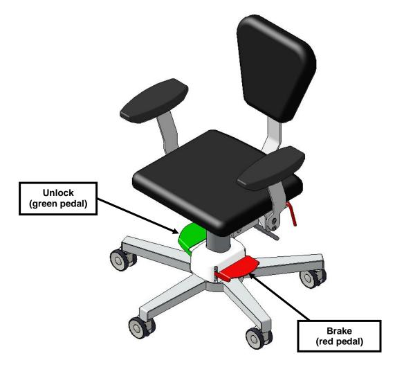
The central locking mechanism is controlled with the pedals located at the base, in the center of the chair. Engage pedal foot pedal in one of the 2 positions:
