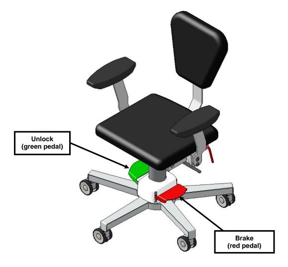
The central brake mechanism is controlled with the pedals located at the base, in the center of the chair. Engage pedal foot pedal in one of the 2 positions:
